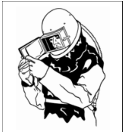
Fig. 3. Exchanging disposable window.
